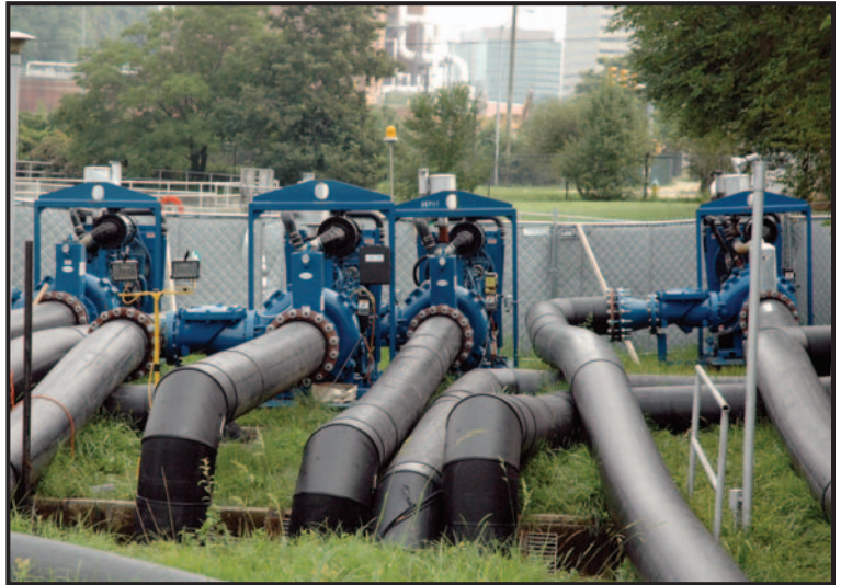
For some applications, such as this job with four 12-inch pumps, you’ll need expert help.
